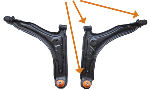
Wishbones have 3 bushings, one on each corner. They all wear out and require changing
