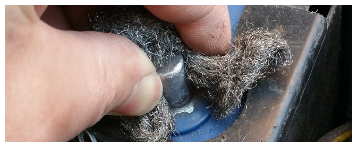
I cleaned up the terminals using wire wool to ensure the contact was good.
