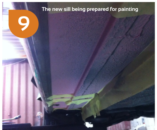
This thick black tar is applied to protect the sill from stone chips and rust
