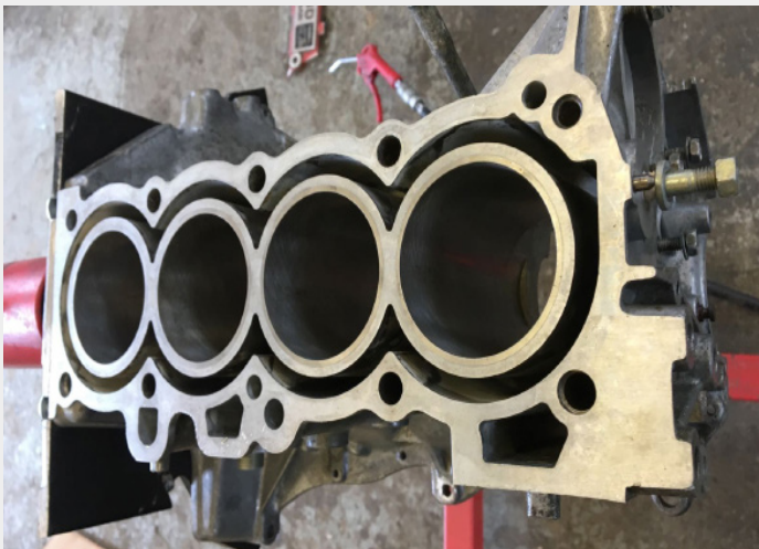
The prepared engine block, awaiting assembly.
