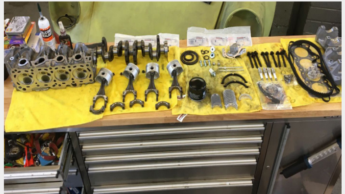
Preparing, cleaning and laying out the parts is essential for an organised build.
