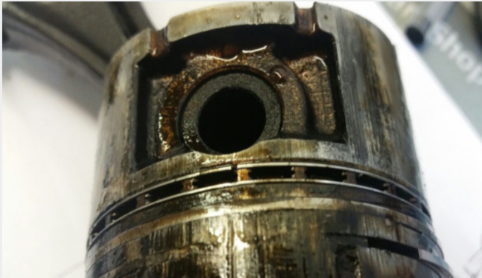
The result of that poor oil, a piston without any cooling. This should be smooth and shiny.
