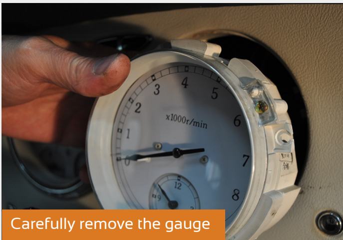
3 x Tabs hold in bezel around the gauge
