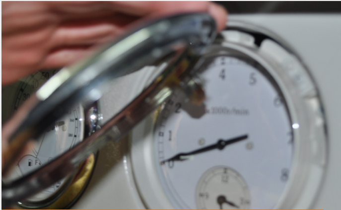
3 x Tabs hold in bezel around the gauge
