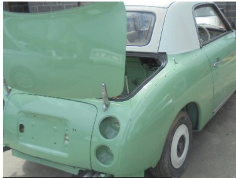
Back half of the car was resprayed
