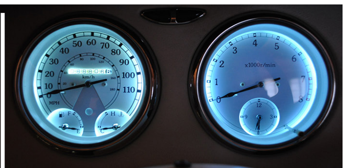
AFTER - NEW LED BULBS FITTED
