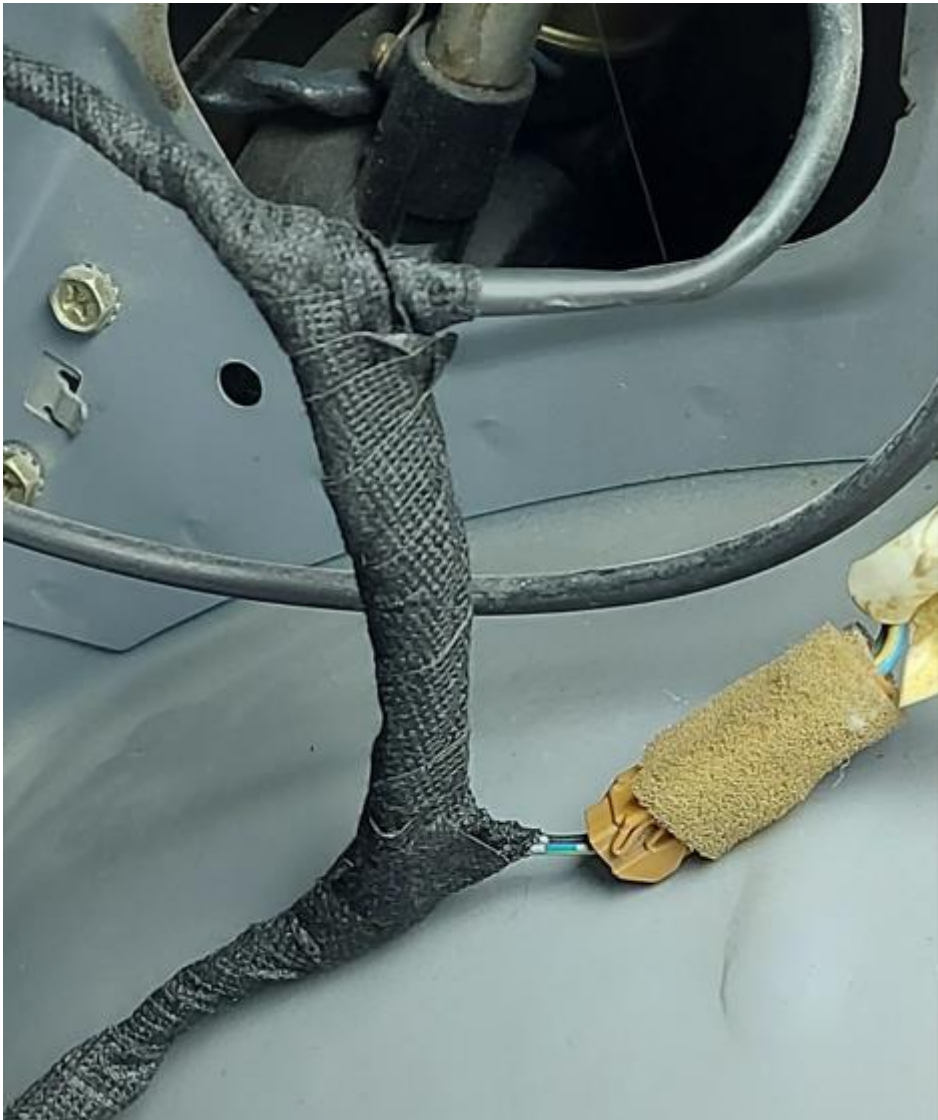
Diode array and connections wrapped with wiring harness tape.
