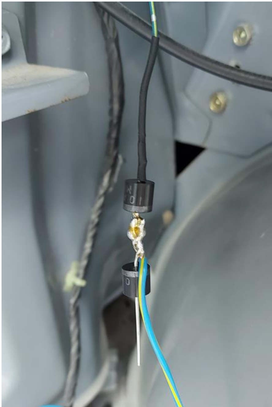
Connection to the hood lock warning C/U Blue & White wire
