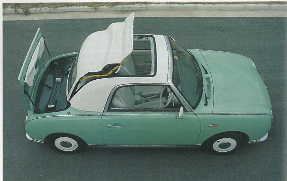
Fabric roof folds away, manually, into a dickey-like hatch; front wings recyclable
